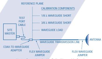
Vector Correction Avoids Bulky Waveguide Coupler
