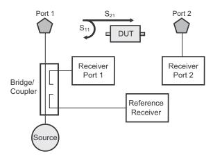
The above illustration is a simplified block diagram of LMR Master's 2-port, 1-path architecture. The magnitude and phase information gained from vector network data enables the LMR Master to make significant error corrections and provide improved field measurements.
