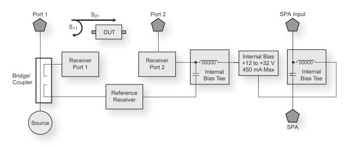
The Compact LMR Master offers optional integrated bias tee for supplying DC plus RF to the DUT as shown in this simplified block diagram.
