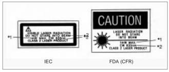
The maximum output is indicated under \*1, and the wavelength under \*2. Caution: Do not look directly into the laser beam.
