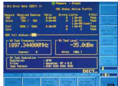
Example of bit error rate measurement (DECT)
