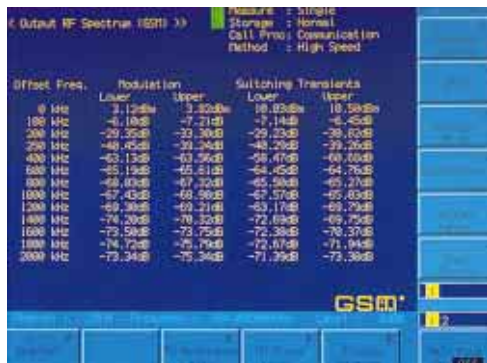
Output RF spectrum measurement (GSM)
