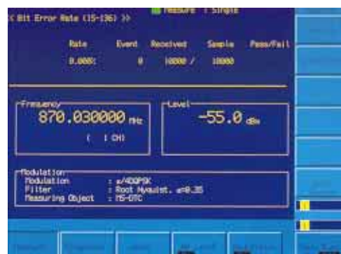
Bit error rate measurement (IS-136A)
