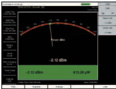
Power Meter measures total input power in a selected frequency span.
