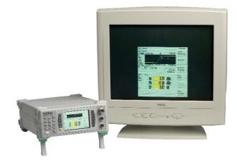
External Video Provides 1/4VGA signal to CRT Monitor
