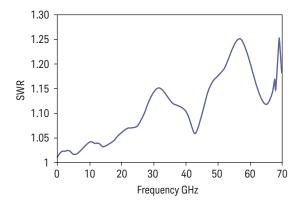
Typical SWR, 10 MHz to 70 GHz (25  $\pm$  10 °C) for N8488A power sensor
