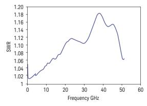
Typical SWR, 50 MHz to 50 GHz (25  $\pm$  10 °C) for N8487A power sensor
