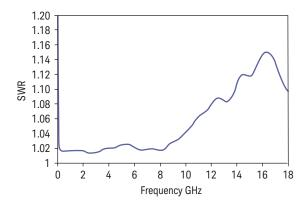
Typical SWR, 10 MHz to 18 GHz (25  $\pm$  10 °C) for N8481A sensor
