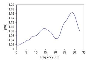
Typical SWR, 10 MHz to 26.5 GHz (25  $\pm$  10 °C) for N8485A sensor
