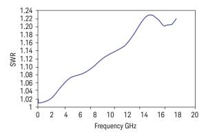
Typical SWR, 10 MHz to 18 GHz (25  $\pm$  10 °C) for N8481H power sensor
