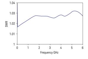
Typical SWR, 100 kHz to 6 GHz (25  $\pm$  10 °C) for N8482A sensor
