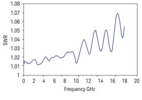
Typical SWR, 10 MHz to 18 GHz (25  $\pm$  10 °C) for N8481B power sensor
