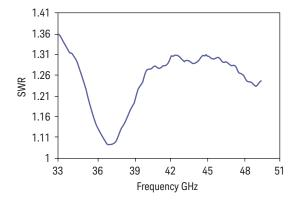
Typical SWR, 33 to 50 GHz (25  $\pm$  10 °C) for N8486AQ power sensor
