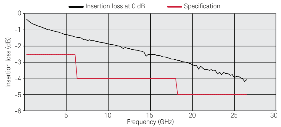
Figure 8. Keysight J7211C attenuation control unit insertion loss (at 0 dB) versus frequency
