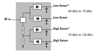
Simplified Block Diagram of Diode-Attenuator-Diode Topology (power levels for "A" suffix sensors)
