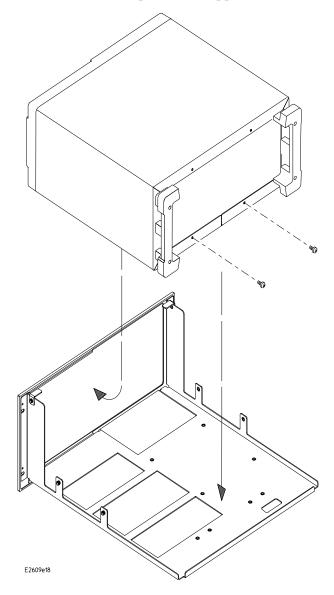
7 Using a T15 TORX screwdriver, install the 2 TORX screws that you removed in step 2, into the rear of the cabinet through the screw holes in the support shelf.
