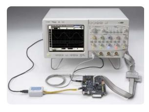
Designing with Altera or Xilinx FPGAs? Use the FPGA dynamic probe for rapid internal FPGA measurements. Using I<sup>2</sup>C, SPI, or CAN? Use the digital channels to acquire and decode these buses, preserving analog channels for other time-correlated measurements.
