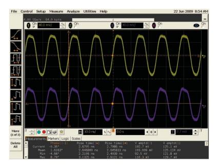
Up to 1 GHz bandwidth and 4 GSa/s high sample rates guarantee you'll see a good representation of the analog characteristics of signals you're testing.
