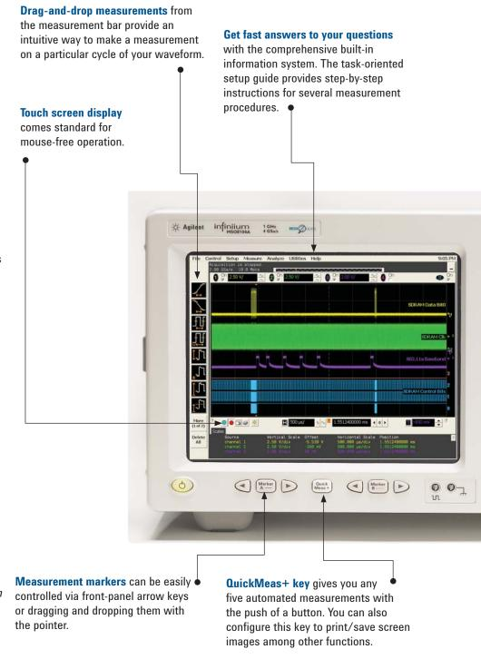
MegaZoom technology enables you to quickly pan and zoom through the deepest waveforms for detailed analysis.
