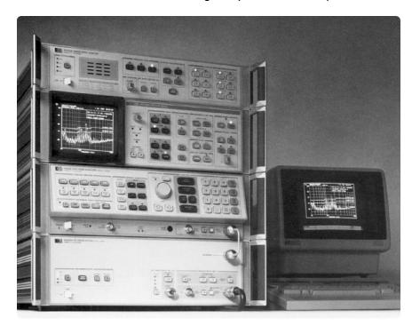
The spectrum analyzer has long burn a useful tool in evaluating electromagnetic interference (EMI) spectra for troubleshooting and preliminary qualification testing. The 8568B spectrum analyzer, with high performance and full programmability, allows difficult and time-consuming EMI compliance tests to be completed automatically.
