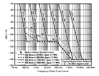
Figure 2. Typical SSB noise versus offset from carrier
