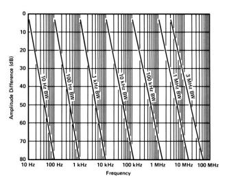
Figure 1. Typical spectrum analyzer resolution
