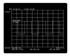
Wide 1 and 3 MHz bandwidths with "Gaussian" shapes improve sensitivity and transient behavior when measuring impulse noise, such as electromagnetic interference, or demodulating wideband spectra.
