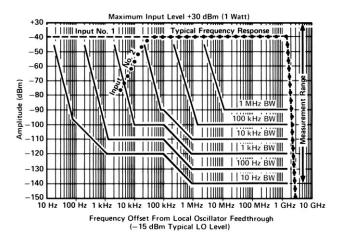
Figure 4. Typical sensitivity vs. input frequency
