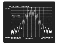
First. press [CENTER FREQUENCY] and position the signal at the center of the screen using one of the data controls (e.g., the knob, step keys, or the numeric keypad).
