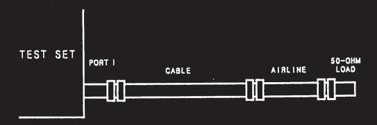
Figure 1. Return Loss Set-up
