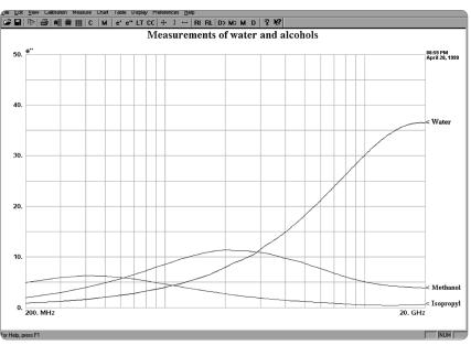
Software displays dielectric constant and loss factor as a function of frequency.
