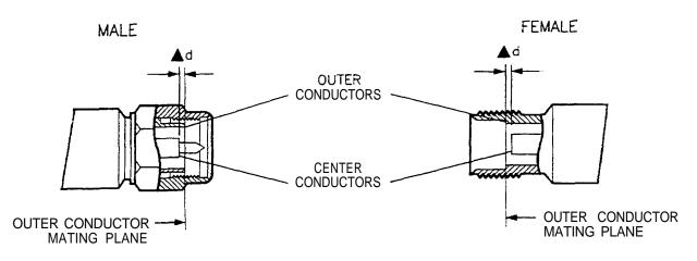
Zero pin depth is when  $\Delta d = zero$ . A protruding center conductor is when  $\Delta d$  is a positive (+) value. A recessed center conductor is when  $\Delta d$  is a negative (-) value.
