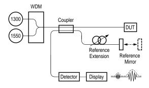
(The 400 mm measurement window can be offset by simply adding length to the reference path at the instrument front panel).
