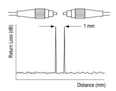
nomenon can be demonstrated with a simple connector pair with an air gap of 1 mm.
