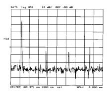
In this measurement, there are several reflections, some which are very small. Through averaging, the measurement sensitivity can be increased. Press **AVG**, [Averaging On], and let the instrument take several sweeps. This allows us to see reflections that may not have been visible before. In this measurement, a fifth reflection is now clearly visible.
