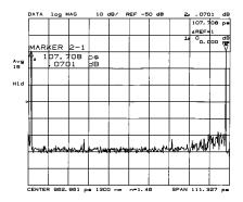
Using the time format, we can now determine the effective delay that one signal path experiences relative to others. With 25 micron two-event resolution, propagation delays as small as 80 femtoseconds can be characterized.
