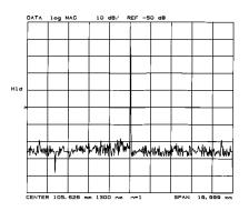
Next, examine the return loss as the second half of the connector pair is mated with the first. As the second ferrule approaches the first, you see two reflections, spaced 2.5 mm apart. The reflection off the second ferrule is low because not all of the reflected light is coupled into the fiber.
