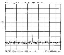
For this particular connector, you not only measure the return loss, by decreasing the measurement span to 1 mm, you measure the gap between the connector ferrules.
