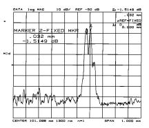
As the connector pair is fully torqued, the two ferrules make physical contact and the two reflections become one. The return loss increases to approximately 40 dB, which is a function of the type of connector tested and its cleanliness.
