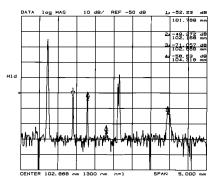
The response between marker 3 and 4 indicates where the back of the ball lens and front of the laser chip meet. Zooming in, we will examine this region.
