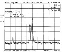
Here we see that there are actually two reflections since there is a small gap between the lens and the laser chip. The size of the gap is 43 microns.
