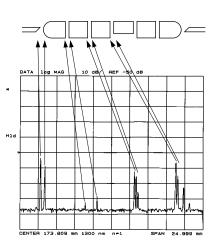
This device has several interfaces, so there are several reflections. The measurement span is 30 mm. The largest reflection, generated from the angled fiber end, is approximately 60 dB. Beyond the Faraday element, there are no reflections, indicating that the isolator is performing its intended function.
