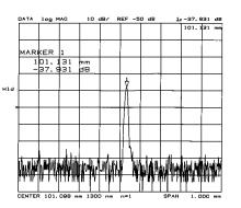
Although this example is of a very simple device, it shows the two basic measurement parameters of the precision reflectometer, specifically high spatial resolution and high dynamic range. The following example shows the usefulness of these measurement capabilities.
