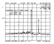
As the two ferrules are brought closer together, the second reflection appears larger as the coupling efficiency increases. Notice also that re-reflections are also seen to the right of the second reflection. The air gap between the two ferrules is now only 32 microns.
