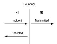
The *reflection coefficient* ' $\rho$ ' of this interface is the ratio of the reflected electric field to the incident electric field and is given by the following:
