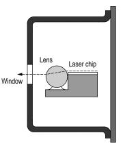
This particular laser module consists of a protective window, a ball lens, and the laser chip. During normal operation of the laser, light propagates from the chip and is focused and aligned through the ball lens before leaving through the window into an attached fiber. Light traveling back into the laser will follow a similar path.
