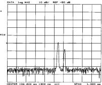
In most applications, the gel termination provides an adequate fiber termination. However, it is not safe to assume that it completely eliminates backreflections.
