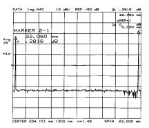
In order to identify each path, we simply terminate one of the ports. As expected, one of the measured reflections will decrease in magnitude thus indicating which response coincides with the terminated port.
