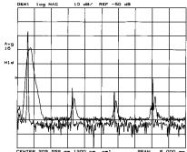
The above plot is a composite measurement of the same device. One measurement is with single mode fiber, while the other is with a 1.25m length of multimode fiber. Each reflection is still visible, and the relative magnitude information is still valid.
