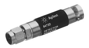
This Planar- Doped Barrier (PDB) detector, combines the best characteristics of point- contact and low barrier Schottky to provide performance never before achievable. This new PDB diode technology provides detectors with broadband-flatness, excellent square-law response, and low SWR.
