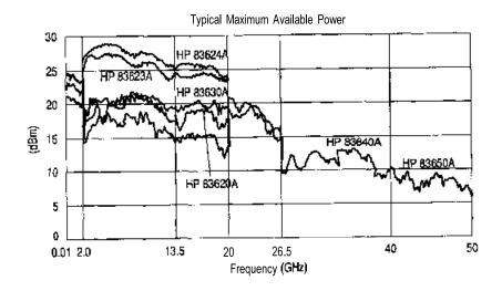
$<sup>^3</sup>$  Specification applies over the 0 to 35°C temperature range (0 to 25°C for output frequencies > 20 GHz). Maximum leveled output power over the 35 to 55°C temperature range typically degrades by less than 2 dB.
