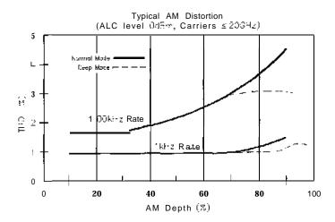
$<sup>^{13}</sup>$  Deep mode offers reduced distortion for very deep AM. Waveform is DC-coupled and feedback-leveled at ALC levels above -13 dBm. At ALC levels below -13 dBm, output is DC-controllable, but subject to typical sample-and-hold drift of 0.25 dB/second.
