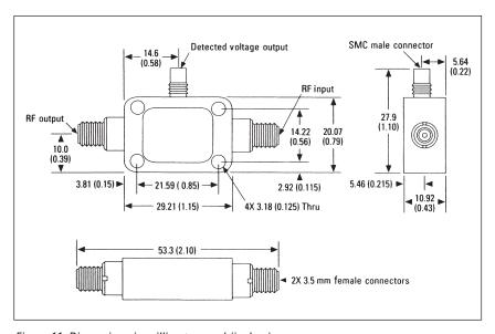
Figure 11. Dimensions in millimeters and (inches)
