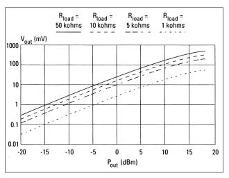
Figure 5. Typical transfer characteristic. Frequency = 18 GHz temperature = +25 °C
