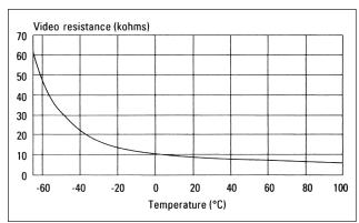
Figure 9. Typical video resistance variation with temperature. Frequency = 18 GHz  $P_{out}$  = -10 dBm
