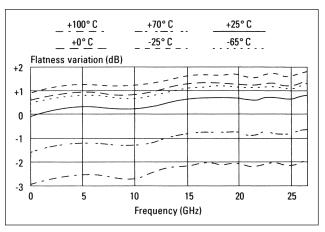
Figure 8. Typical flatness at various temperatures.  $R_{load}$  = 100 k  $\Omega$
