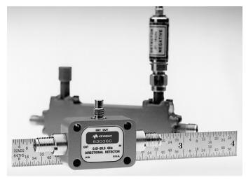
The 83036C is much smaller than the directional coupler-detector combinations which it is designed to replace. The entire unit occupies a volume of less than 0.47 cubic inches (< 8 cm³) vs. a typical connectorized detector which alone can occupy more than 1 cubic inch (16.4 cm³). The directional detector features 3.5 mm microwave connectors and an SMC connector at its dc output.
