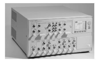
Agilent's 8159xB modular optical switches route light in single mode and multimode optical fibers.
