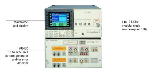
71612C consists of the 70843C 0.1 to 12.5 Gb/s pattern generator and/or error detector with a mainframe/display and optional clock source
