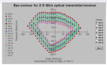
Use HP E4543A application software to derive eye contours to  $10^{\cdot 20}$  BER from  $\,$  Q measurement.
