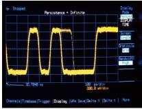
See captured errored bit on an oscilloscope.
