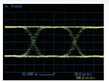
Fast transition time and low jitter of the data output eye diagram at 12 Gb/s.
