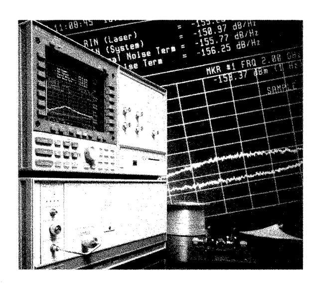
The HP 71400C and 71401C lightwave signal analyzers combine HP's highest-performance RF spectrum analyzers with a sensitive, wide-bandwidth optical-receiver for analyzing lightwave communications systems and components.
