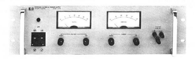
Figure 1-1. Model 6439B DC Power Supply
