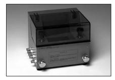
DUT Connection: 2-Terminal Bias Voltage Output connector: BNC(f) Dimensions (approx.):  $216(W) \times 173(H) \times 235(D) \text{ [mm]}$  Weight (approx.): 2500 g Basic Measurement Accuracy:  $2\%(<1 \text{ kHz}), 1\% \ (\ge 1 \text{ kHz}), 2\% \ (>1 \text{ MHz})$  For detailed information, refer to the operation manual of 42841A.
