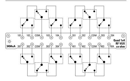
The 34941A and 34942A are configured as four independent 1x4 RF multiplexers on a single module. Multiple banks can be connected together to create a larger multiplexer. To prevent ground loops, individual multiplexers are isolated from each other and from the mainframe's chassis. However, the multiplexer channels can be chassis grounded with a simple change. Both 50-ohm and 75-ohm versions are available.
