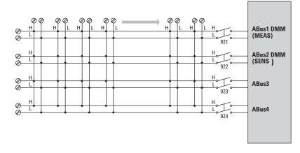
Note: The 34933A has 100 ohm input protection resistors to limit current and protect the reed relays.
