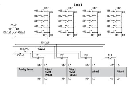
Figure 4. 34925A 40/80-channel optically isolated FET mux (shown in 1-wire mode bank 2)
