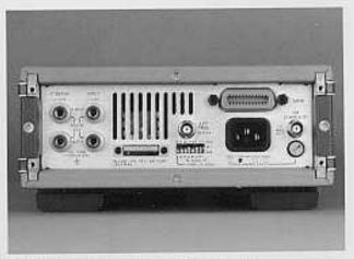
Switchable rear inputs and synchronizing signals.
