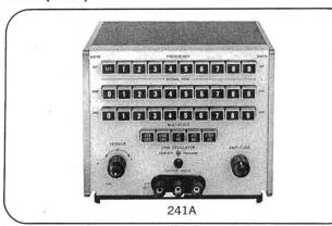
Any frequency between 10 Hz and 999 kHz can be selected to three significant figures by simply pushing the three appropriate frequency pushbuttons and one of five decade multipliers. These pushbuttons control 900 base frequencies in increments of 0.1 Hz from 10.0 to 99.9 Hz, providing 4500 discrete frequency settings. Infinite resolution is provided by a vernier control, extending the upper frequency to 1 MHz.
