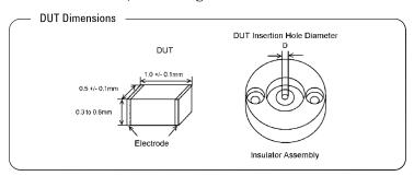
The 16196B is furnished with three different insulator assemblies, since any gaps between the DUT and the cylindrical insulator will result in improper positioning and subsequent measurement errors. Select an insulator assembly that reduces the gap the most. See the table below for dimensions of the insulator assemblies.
