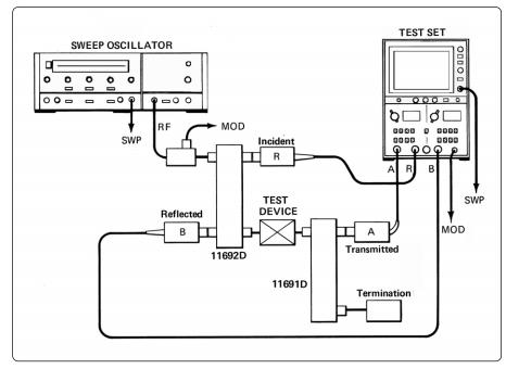
Figure 1. Setup for simultaneous swept measurement of insertion loss (A/R) and return loss (B/R), using 11691D and 11692D couplers.
