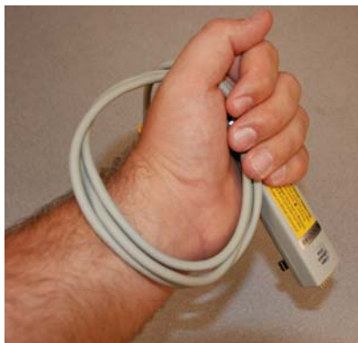
Figure 6 Recommended Coil for Storage
