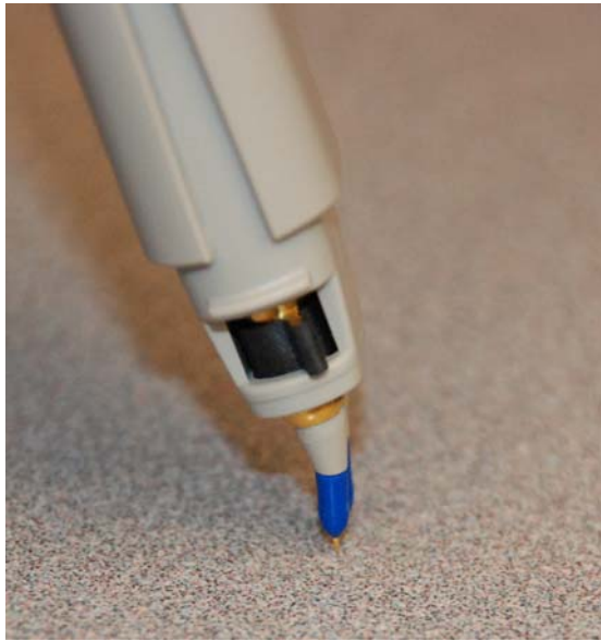
Figure 21 Proper Vertical Orientation of the Blue Tips
