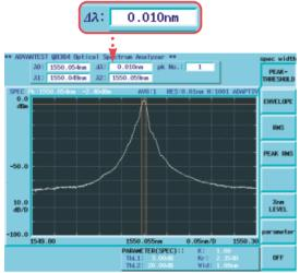
FIG. 1 Resolution band width of 10 pm
