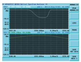
FIG. 13 Upper: measuring signal, 2 nm SPAN. Lower: reference signal, 30 nm SPAN Although prior measurement systems required that reference and measuring signals be put under the same conditions, the Q8384 enables measurements even if these signals are under different conditions.
