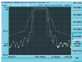
FIG. 17 Limit line function
