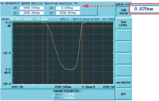
FIG. 14 Notch filter: wavelength width at 3 dB loss
