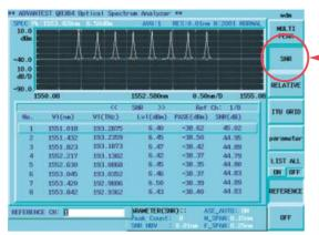
FIG. 8 SNR display Wavelength-specific S/N ratio measurements are displayed.
