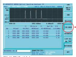
FIG. 10 ITU-T grid display
