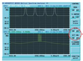
FIG. 11 WDM alternate sweeping Upper: 5 nm SPAN, Lower: 50 nm SPAN
