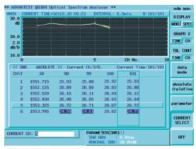
FIG. 20 WDM monitor (SNR mode) SNR display with channel No. on the horizontal axis (with limit line)
