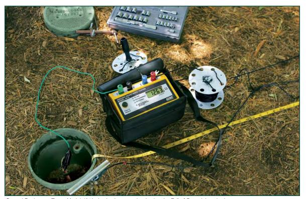
Ground Resistance Tester Model 4610 checks the ground rod using the Fall-of-Potential method.
