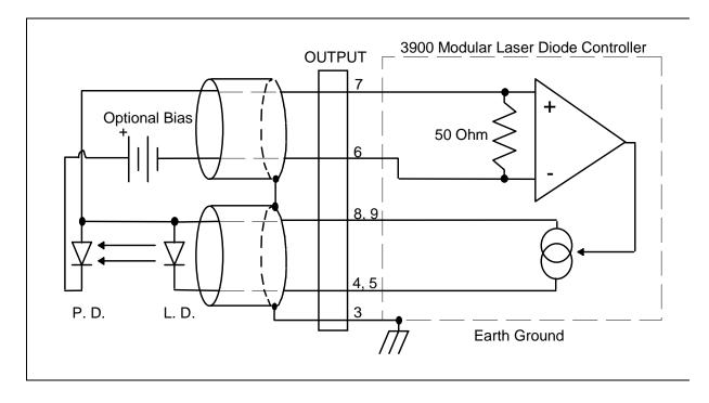
Figure 2.6 Common Laser Anode - Photodiode Anode
