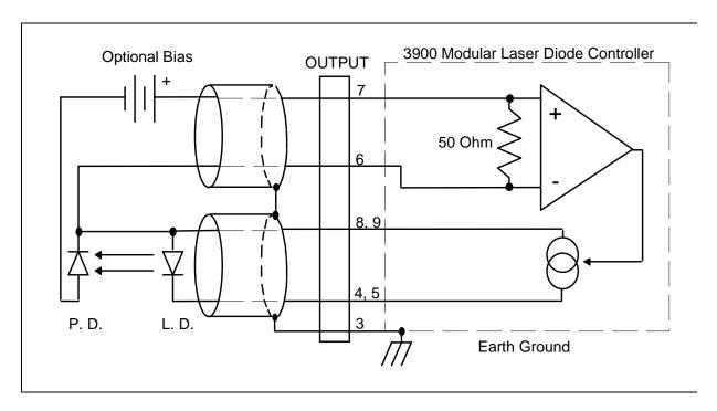
Figure 2.5 Common Laser Anode - Photodiode Cathode
