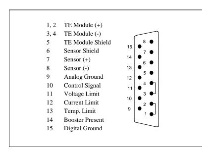
Figure 2.7 Back Panel TEC Connector
