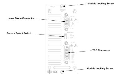
Figure 2.1 LCM-39420 Back Panel
