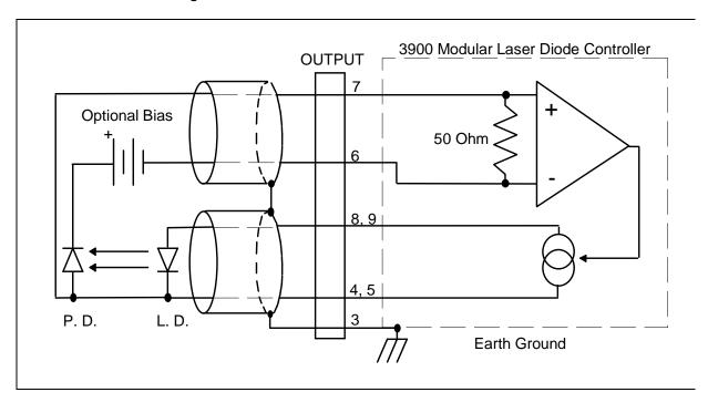
Figure 2.4 Common Laser Cathode - Photodiode Anode
