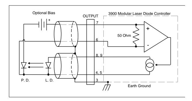
Figure 2.3 Common Laser Cathode - Photodiode Cathode
