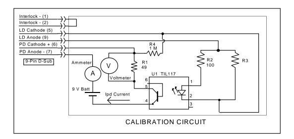
Figure 3.1 I<sub>PD</sub> Calibration Circuit
