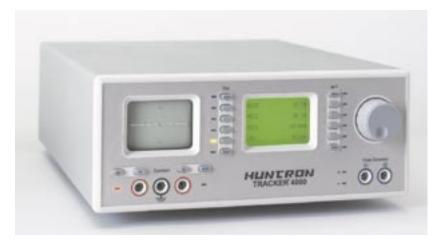
The Huntron® Tracker® 4000 provides state-of-the-art troubleshooting methodology using analog signature analysis techniques. The dual trace CRT display quickly compares known good component signatures with the device under test, thus detecting subtle problems such as IC leakage, intermittent faults, open capacitors etc. All this and more without the need to power up the circuit under test and perhaps cause further damage.
