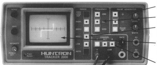
Advanced pulse generator for testing gatefired devices.
