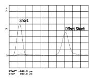
Accurately evaluate the response of your device in the time domain by removing the dispersive effects of the waveguide.
