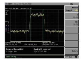
The occupied bandwidth is measured in dBc.
