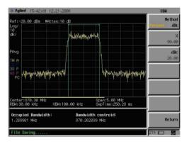
The occupied bandwidth is measured in percentage.
