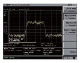
Center frequency, main channel bandwidth, adjacent channel bandwidth, and channel space can be set on the panel.
