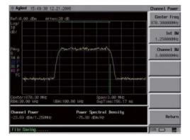
It is quick and easy to set center frequency, integration bandwidth, and channel bandwidth on the panel.
