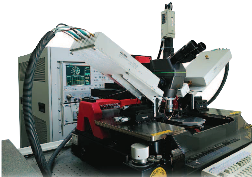
On-wafer measurements to 110 GHz with the ME7808B
