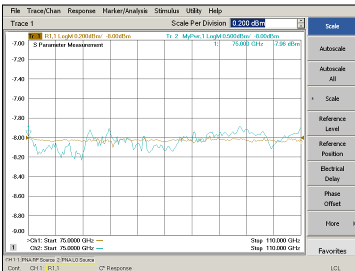
Figure 1. A demonstration of power accuracy; power sensor measurement vs. N5247A PNA-X R1 receiver < 0.1 dBm
