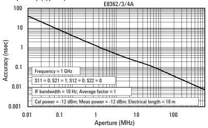
In general, the following formula can be used to determine the accuracy, in seconds, of a specific group delay measurement:
