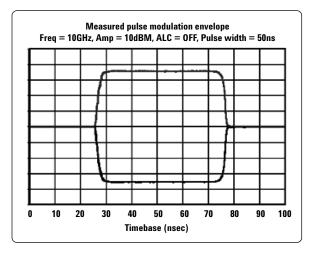
With ALC off, specs apply after the execution of power search. For instruments without a step attenuator, specs apply between 0 and +10 dBm. For instruments with the step attenuator, specs apply with Atten Hold Off, or ALC level between 0 and +10 dBm.
