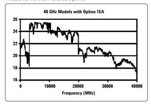
(Same as max power sweep range) From -20 dBm to maximum specified output power with step attenuator in 0 dB position. Can be offset using Option 1E1 attenuator.
