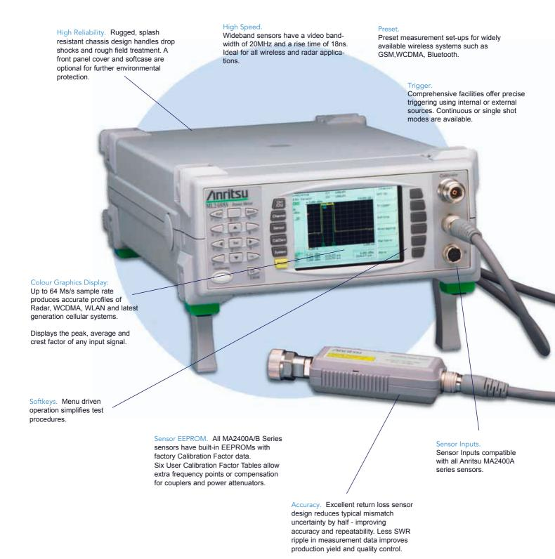
The dual display channel gives complete flexibility and can provide two different perspectives on the measurement.
