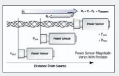
Standing waves are created when impedance mismatch causes RF signal reflections. The magnitude of the standing wave varies along the transmission line as the incident signal and reflected signal add and subtract vectorially.
