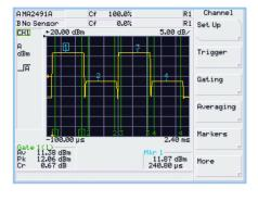
The graphical display and the measurement gate makes the measurement of GSM and PCS systems straightforward.
