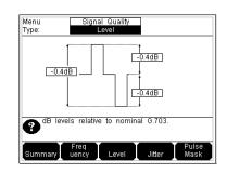
Easily identify any frequency, level, pulse shape or jitter problems.
