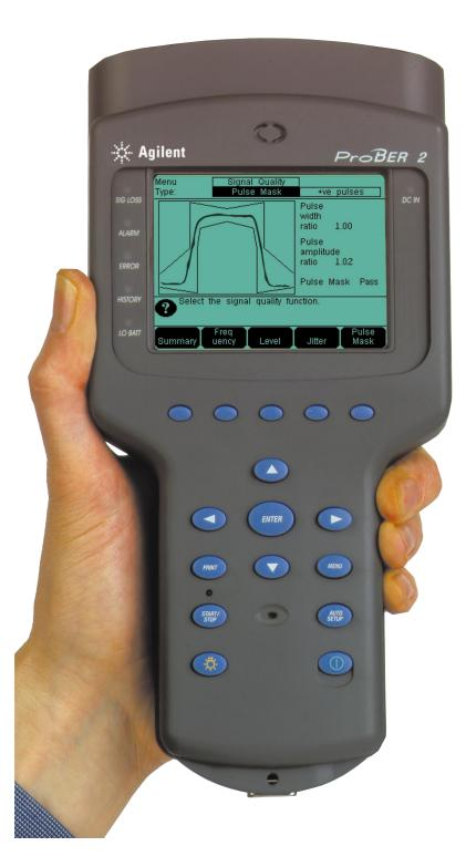
The ProBER 2 test set provides a powerful handheld solution for testing 2 Mb/s and 64 kb/s digital circuits. It offers extensive BER test functions plus a unique range of signal quality measurements (pulse mask, jitter, level and frequency). This unmatched test capability, combined with the intuitive operation of ProBER 2, simplifies installation and maintenance testing for faster problem resolution.
