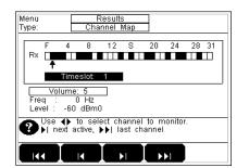
At-a-glance display of active timeslots, frequency and level measurements combined with the ability to listen to timeslots.
