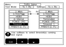
Single transmit/receive setup display minimizes the number of key presses and lets you see the instrument configuration at a glance.
