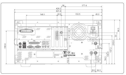
Figure 1-3. Dimensions (side view, in millimeters, nominal)
