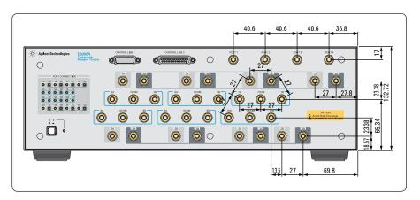
Figure 3-3. Dimensions (rear view, with Option E5092A-020, in millimeters, nominal)
