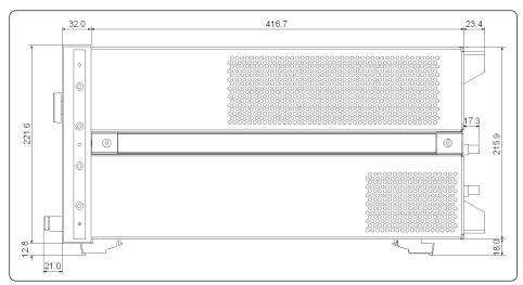
Figure 1-4. Dimensions (top view, in millimeters, nominal)
