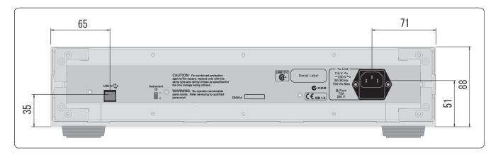
Figure 2-4. Dimensions (side view, with Option E5091A-009, in millimeters, nominal)
