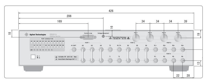
Figure 2-3. Dimensions (rear view, in millimeters, nominal)
