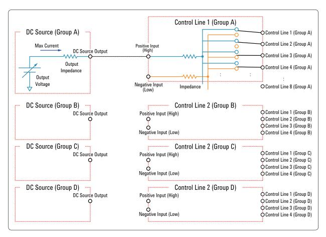
Figure 3-7. Control line pin assignment (E5092A-020)
