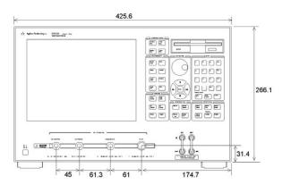
Figure 1-5. Dimensions (front view, in millimeters, nominal)
