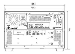
Figure 1-6. Dimensions (rear view, in millimeters, nominal)
