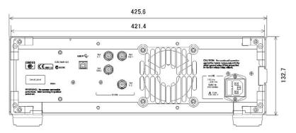
Figure 2-5. Dimensions (rear view, in millimeters, nominal)
