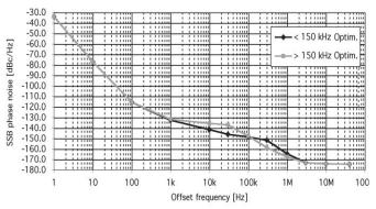
Figure1-4. SSB phase noise sensitivity of different LO optimization (typical)( standard, correlation = 1, carrier frequency = 1 GHz, start offset frequency = 1 Hz, +5 dBm input, measurement time = 17.7 sec)
