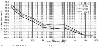
Figure 2-3. E5052A downconverter L0 phase noise (typical)
