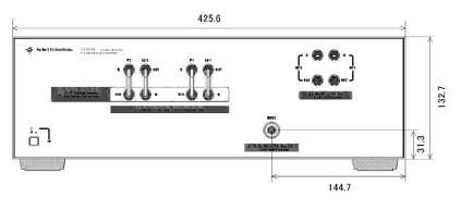
Figure 2-4. Dimensions (front view, in millimeters, nominal
