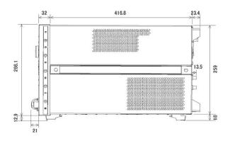
Figure 1-7. Dimensions (side view, in millimeters, nominal)
