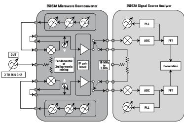
Figure 2-1. E5053A with E5052A block diagram
