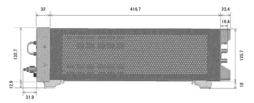
Figure 2-6. Dimensions (side view, in millimeters, nominal)
