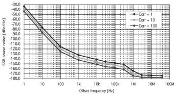
Figure1-3. SSB phase noise sensitivity improved with the crosscorrelation function (typical) (standard, improvement with the correlation, carrier frequency = 1 GHz, < 150 kHz optim., +5 dBm input)
