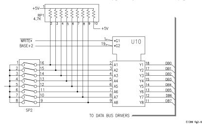
Figure 2-9. Device Type Register
