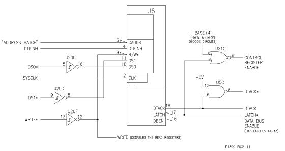
Figure 2-11. DTACK Circuitry
