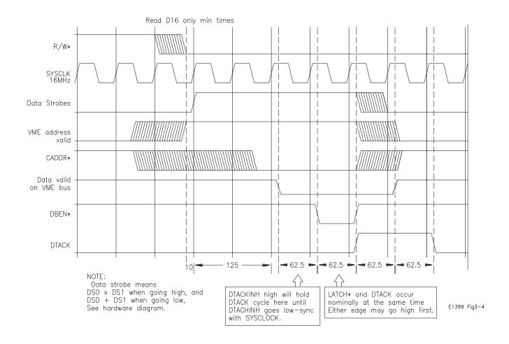
Figure 3-4. Timing for Writing to the Control Register
