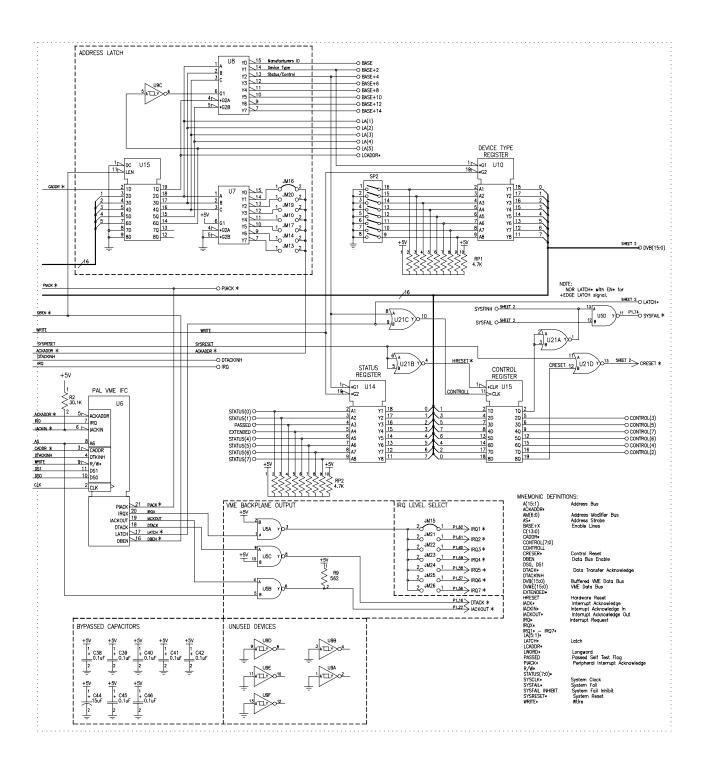
Figure B-1. HP E1399A Breadboard Schematic (2 of 2)
