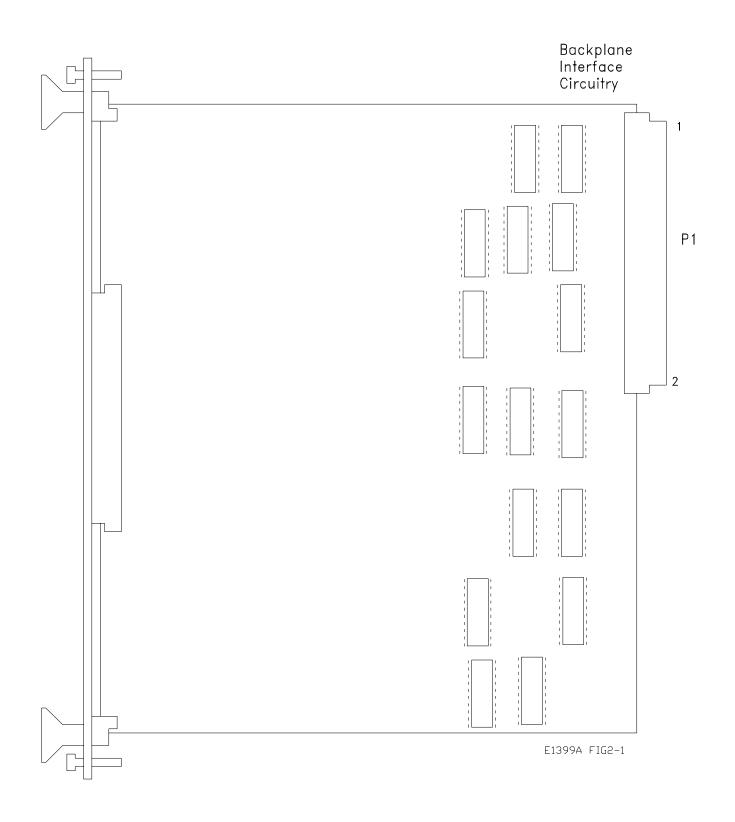
Figure 2-1. HP E1399A Breadboard Module & Connector Pinout
