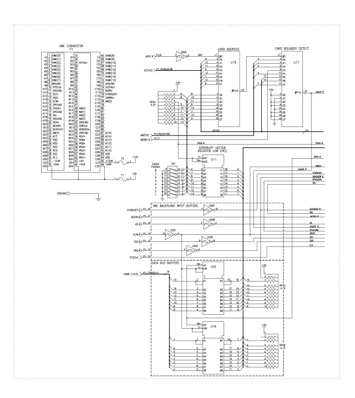
Figure B-1. HP E1399A Breadboard Schematic (1 of 2)
