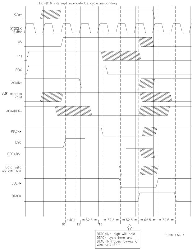
Figure 3-5. Interrupt Timing
