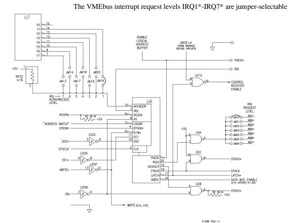
Figure 2-12. Interrupt Circuitry
