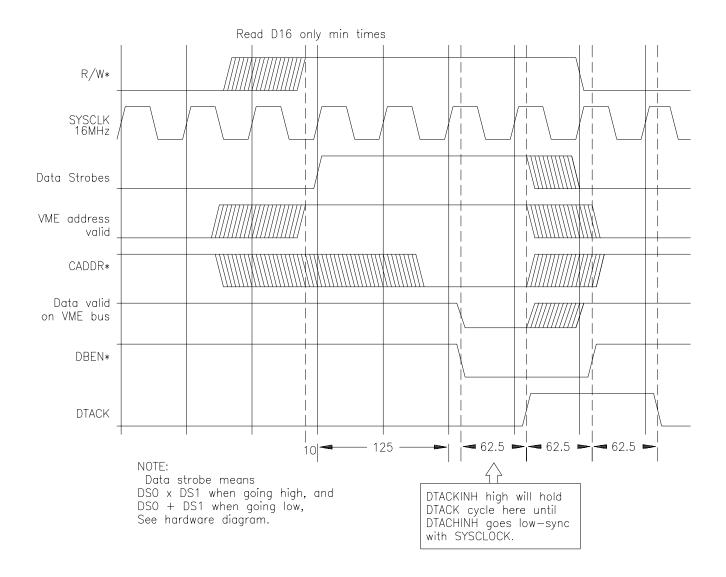
Figure 3-2. Timing for Reading the Status Register
