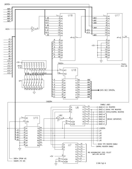
Figure 2-6. Address Lines and Register Decoding
