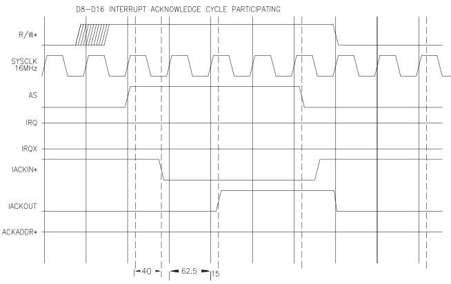
To meet VME timing spec, an external IACKOUT disable is also used.
