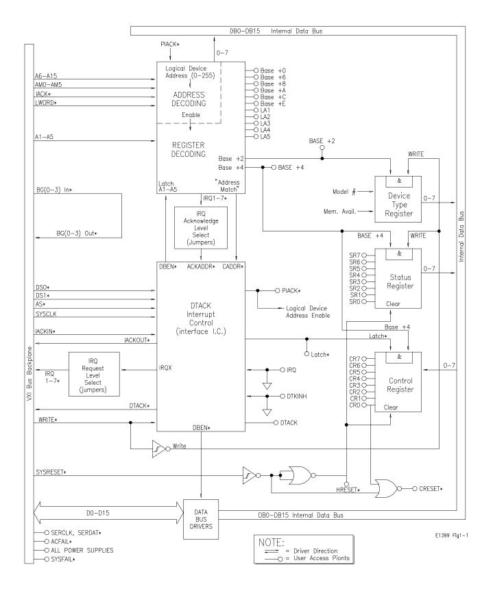
Figure 1-1. Digital Backplane Interface Block Diagram
