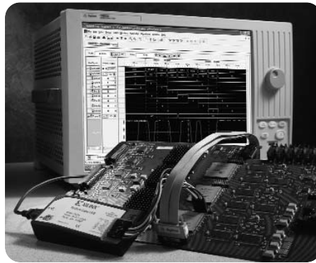
Figure 1. The FPGA dynamic probe application endows your logic analyzer with unique productivity enhancements to find problems more quickly.
