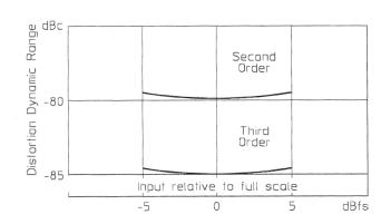
Typical harmonic and intermodulation distortion
