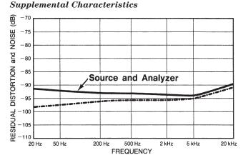
Typical residual distortion and noise of the source and analyzer combined (source voltage set to 1.5 V, 80 kHz BW). Dashed line represents typical residual distortion and noise for the analyzer only.
